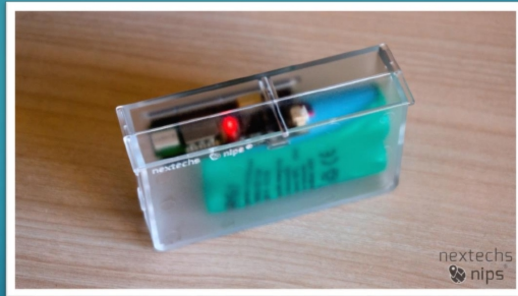
NIPS TAG encased in a plastic box with a 6400 mAh Lithium battery
